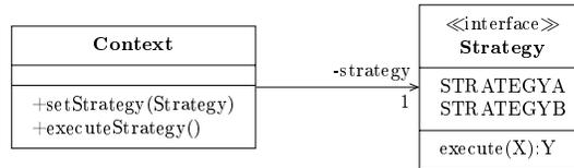
Figure 3: The strategy pattern, functions defined in a functional interface (listing 5)
