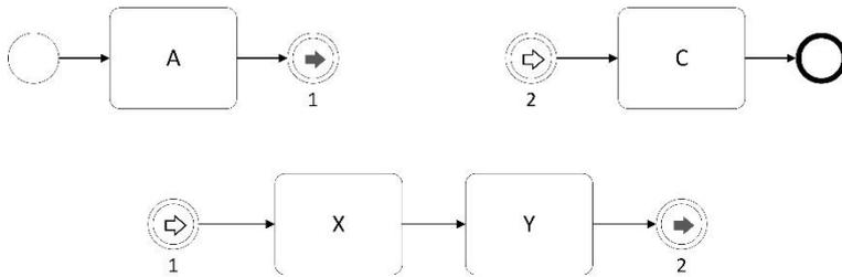
Figure 3 - Horizontal modularization (Winter et al., 2020)
