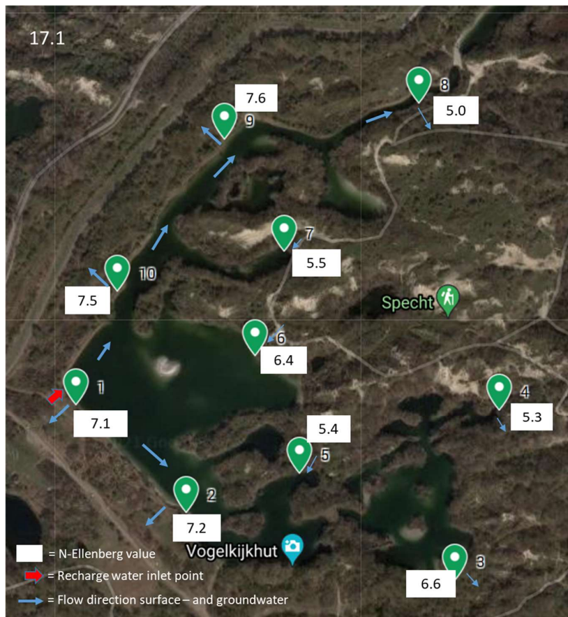
Figure 5 Pond 17.1 With Flow Directions of Surface – and Groundwater
