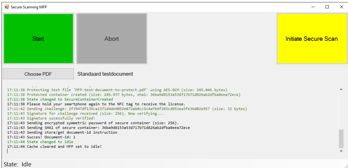
Figure A.7: MFP prototype, document hash and key communicated with smartphone
